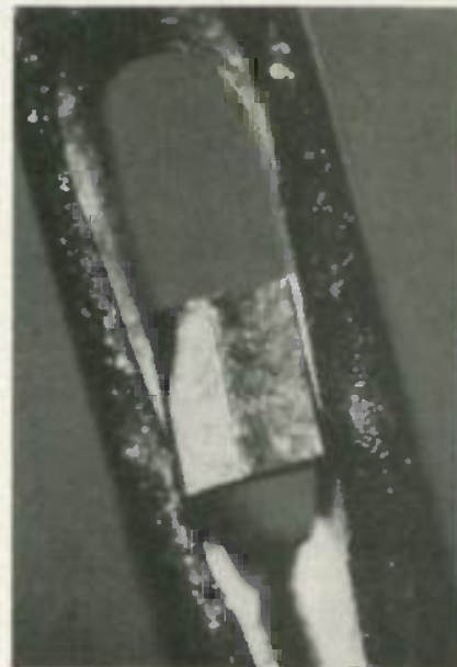
FIG. 4—THIS SEMICONDUCTOR LASER is so tiny that it can fit in the eye of an ordinary sewing needle. Photo courtesy of ATT Bell Laboratories.
