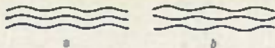
FIG. 3—IN LASER LIGHT, all of the waves are in phase; thus they are said to be coherent (a). In normal light, the waves have no phase relationship (b).
