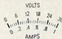
FIG. 8—ENLARGE OR REDUCE THIS METER SCALE to fit the meter you use, and then glue our scale over yours.
