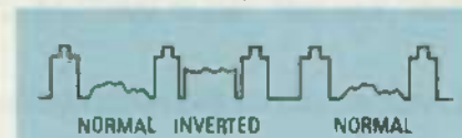
FIG. 2—IN SOME SCRAMBLING SYSTEMS the polarity of the video alternates every frame or every few frames.
